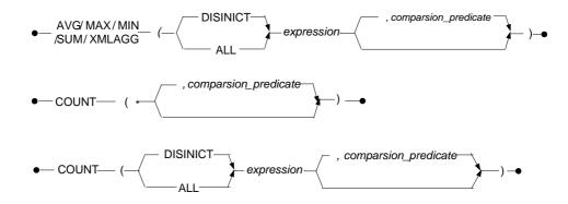
Figure 3-125 AGGREGATE FUNCTION syntax
