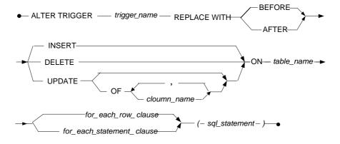
Figure 3-25 ALTER TRIGGER REPLACE syntax
