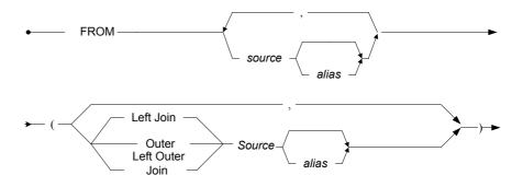
Figure 3-115 DBMaker Outer-Join Syntax
